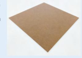
Prototype MDF that used a wood-derived adhesive
