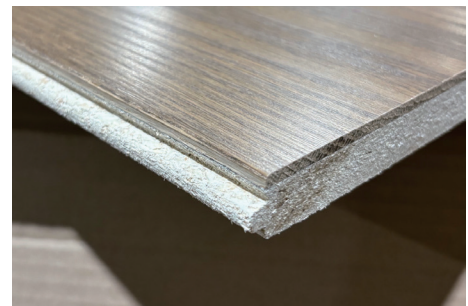
An image of using "DIO woodcore" for the flooring substrate
