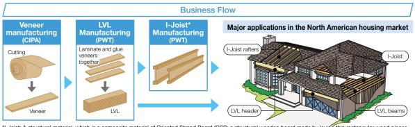
\*I-Joist: A structural material, which is a composite material of Oriented Strand Board (OSB: a structural wooden board made by laying thin rectangular wood pieces cut from raw wood upon one another in such a way that the surface layer and core layer cross at right angles in the fiber direction and are then compressed at high temperature), LVL, and timber.
